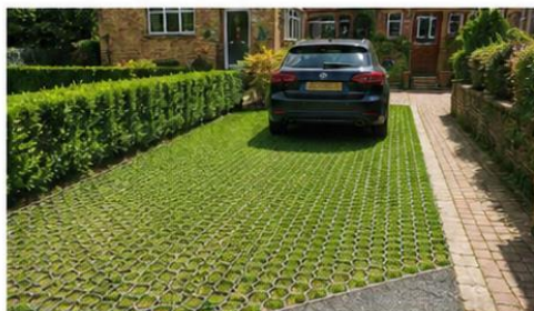
Figure 3: Example of Reinforced Grass Driveway in Use
