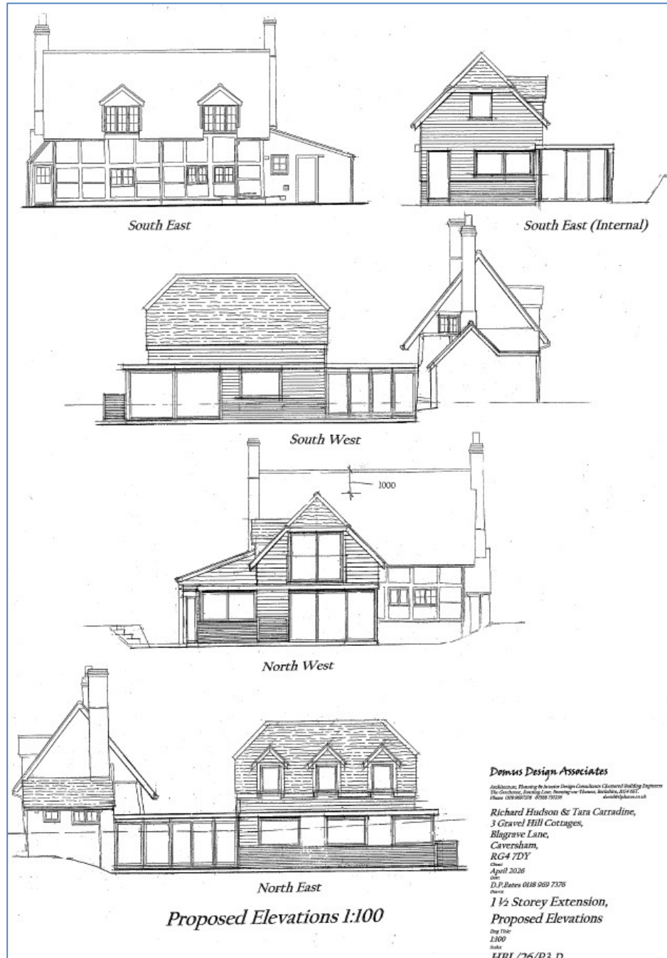
Fig. 22 Elevations of the proposed extension (existing ground level shown as dashed line on SW/NE elevations). OS PMCL AC0000855630
