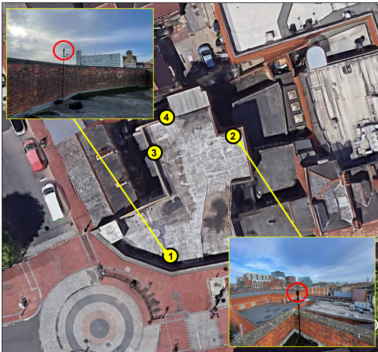
Figure 3 Noise survey measurement locations (Image Reference: Google Earth)
