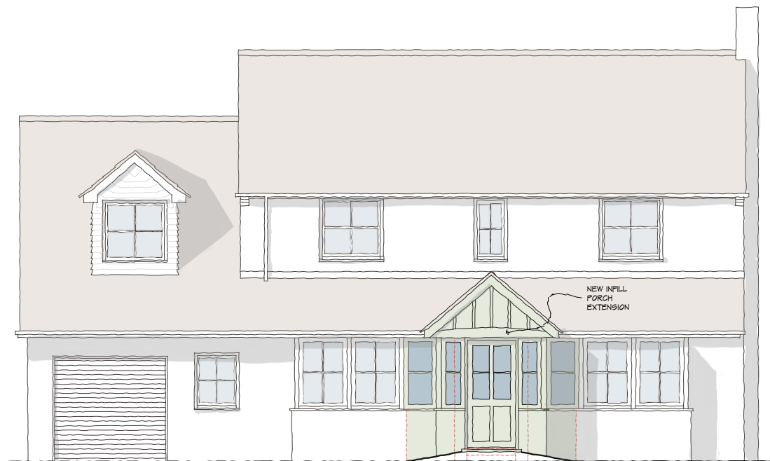
FRONT ELEVATION SOUTH WEST - 1:100
