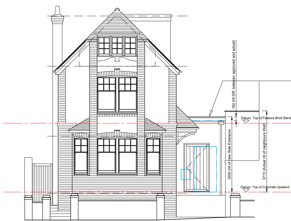
FRONT ELEVATION As Constructed Scale 1:100
