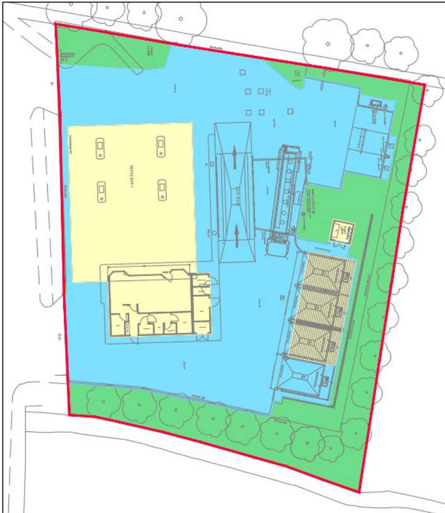
Figure 3-2 – Drained Areas Analysis Extract – Post-Development
