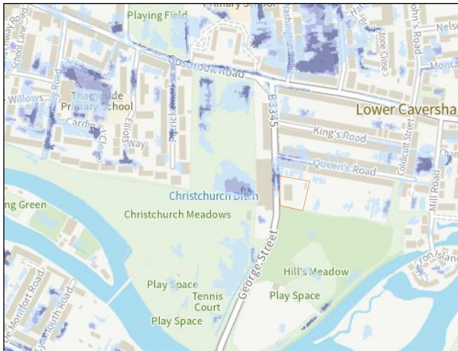
Figure 4-2 – Extract of the Environment Agency's Long Term Surface Water Flood Risk Mapping (including climate change allowance)
