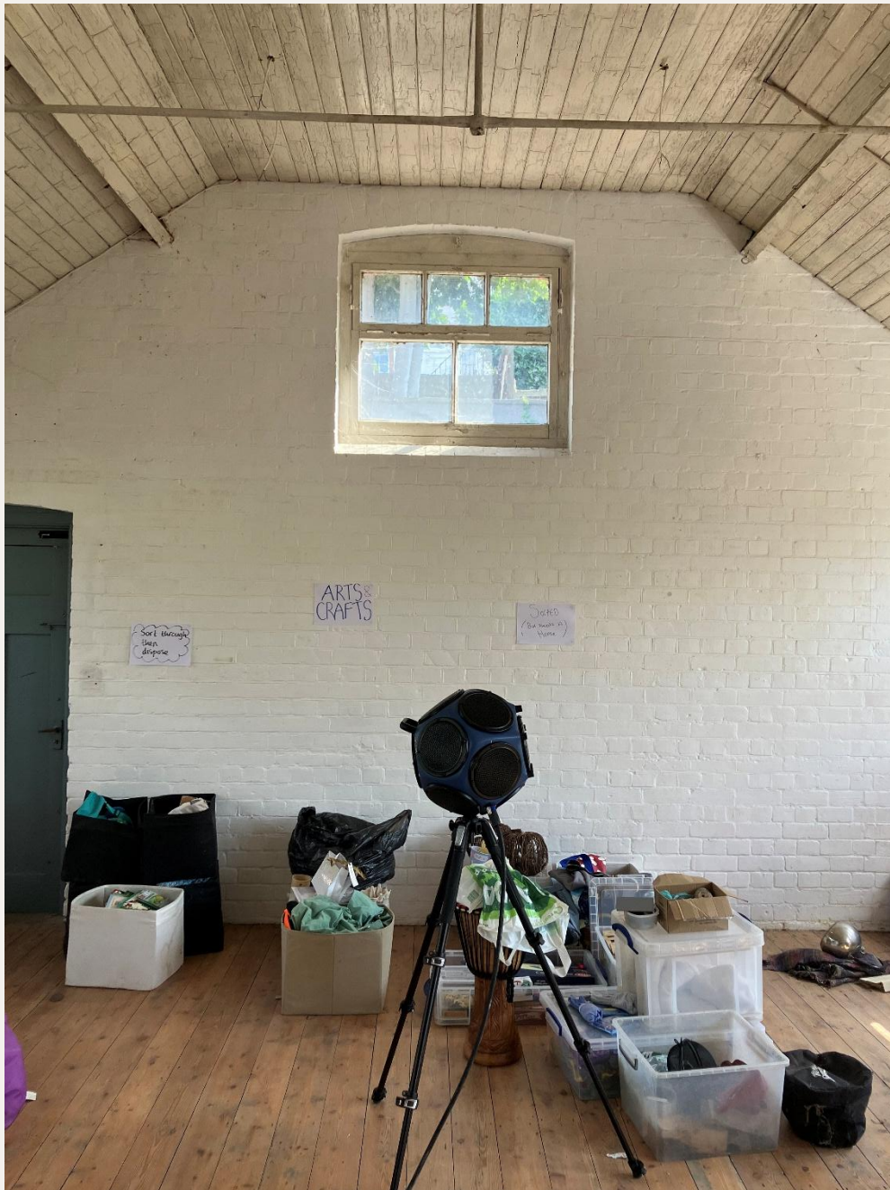
Figure 3-8 Photograph showing dodecahedron loudspeaker in position 2
