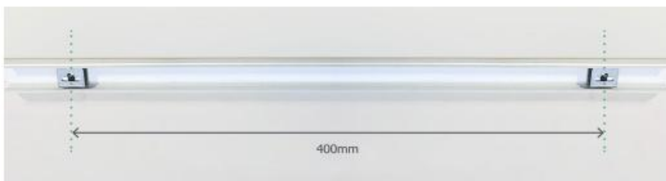
400mm gap is left between D-clip centres
