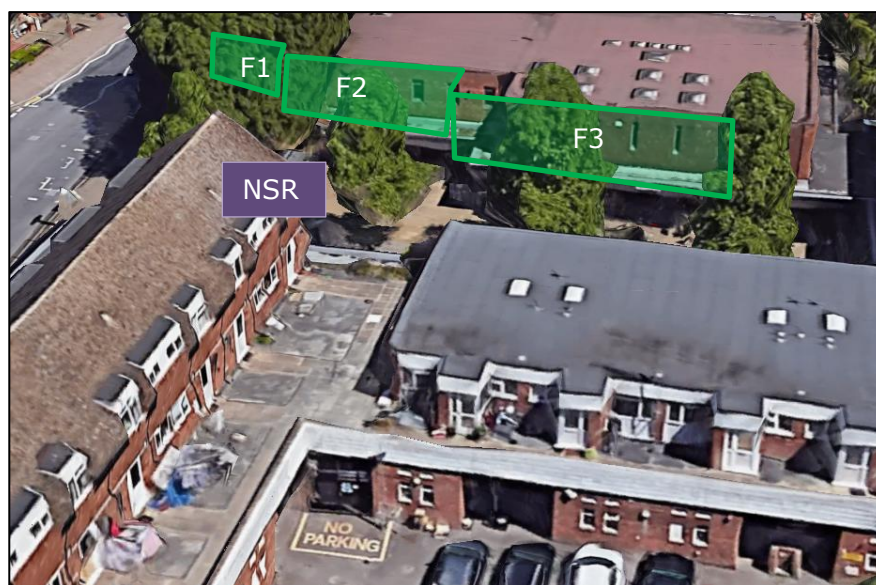
Figure 4: 3D view showing the proposed gym and fitness venue, the closest noise-sensitive receptor (NSR) and the façade elements considered within the breakout noise assessment. The coloured façade areas indicated F1, F2 and F3 are the building elements included within the noise propagation calculations
