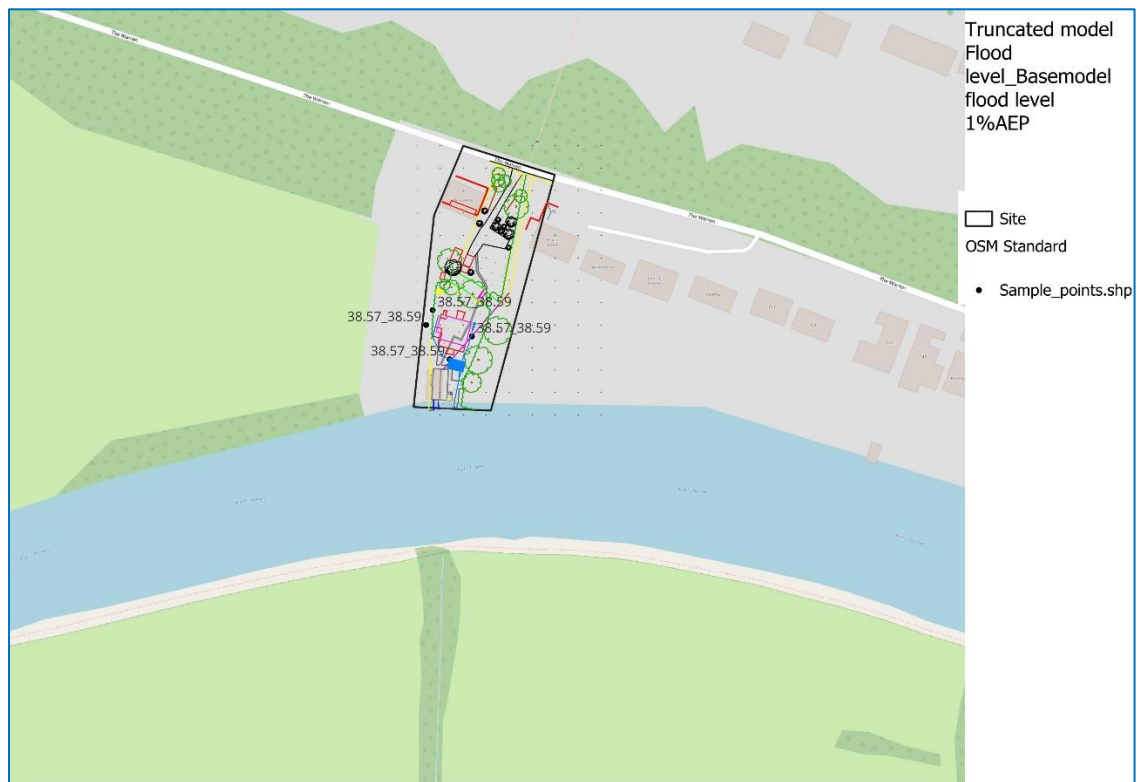
Figure 4 : Validation of Truncated model flood levels to original model at the site
