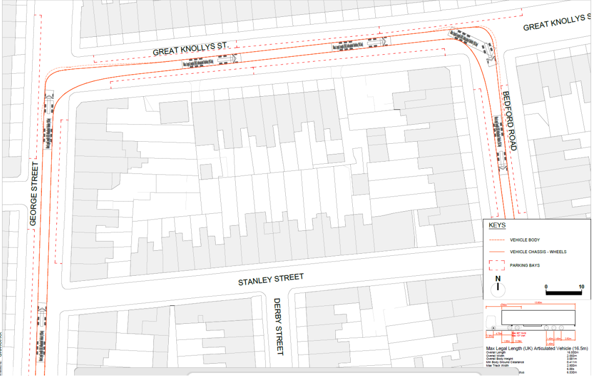
SWEPT PATH ANALYSIS - 16.50M ARTICULATED VEHICLE EGRESS
