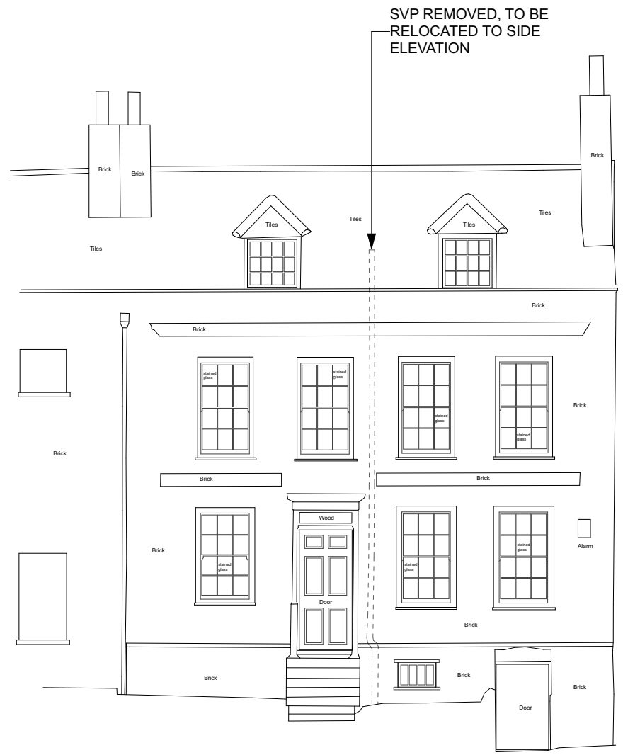
EXISTING FRONT / EAST ELEVATION 1:100
