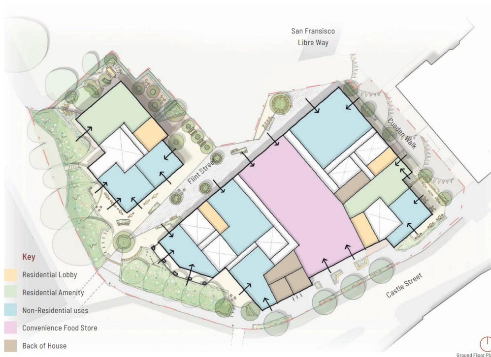
Figure 4 Mixed Ground Floor Uses
