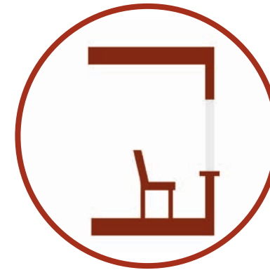
Avoidance of Full Height Windows Orientation specific glazing ratios to limit overheating risk.
