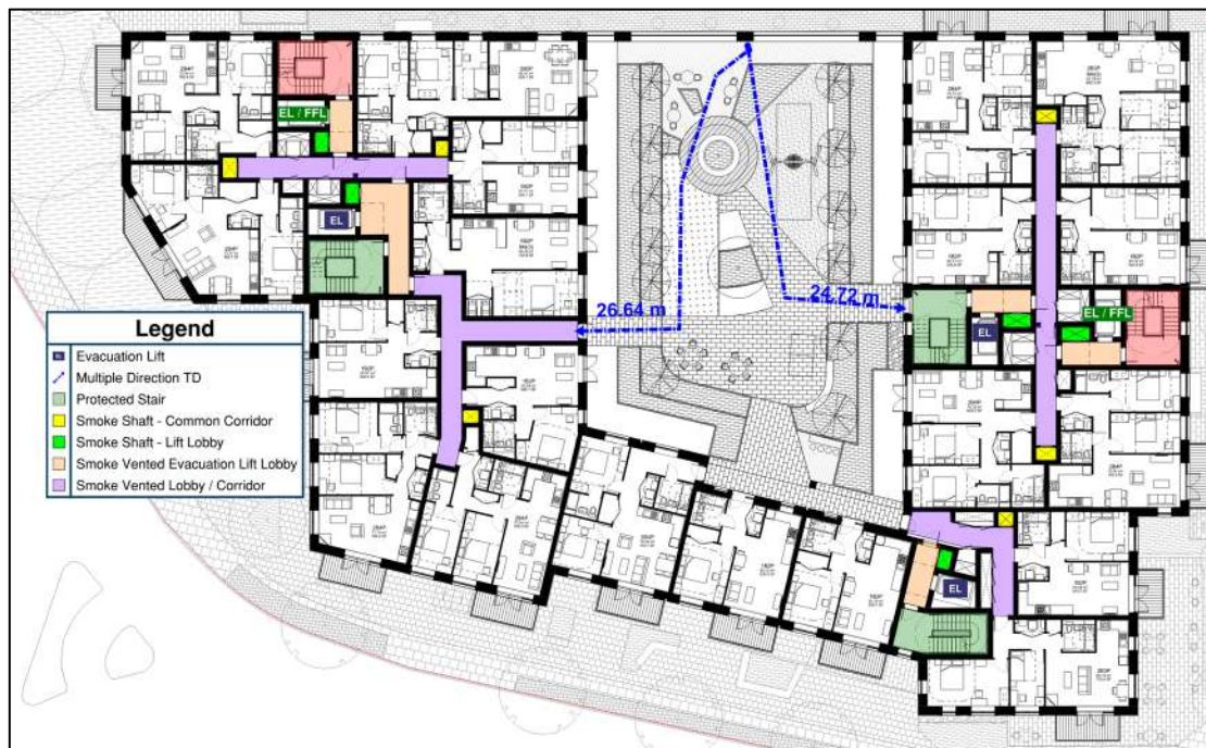
Figure 10 – Roof Terrace Travel Distance – Block A Level 01
