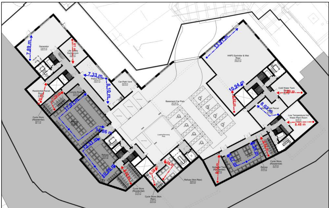
Figure 9 – Basement Level Travel Distances
