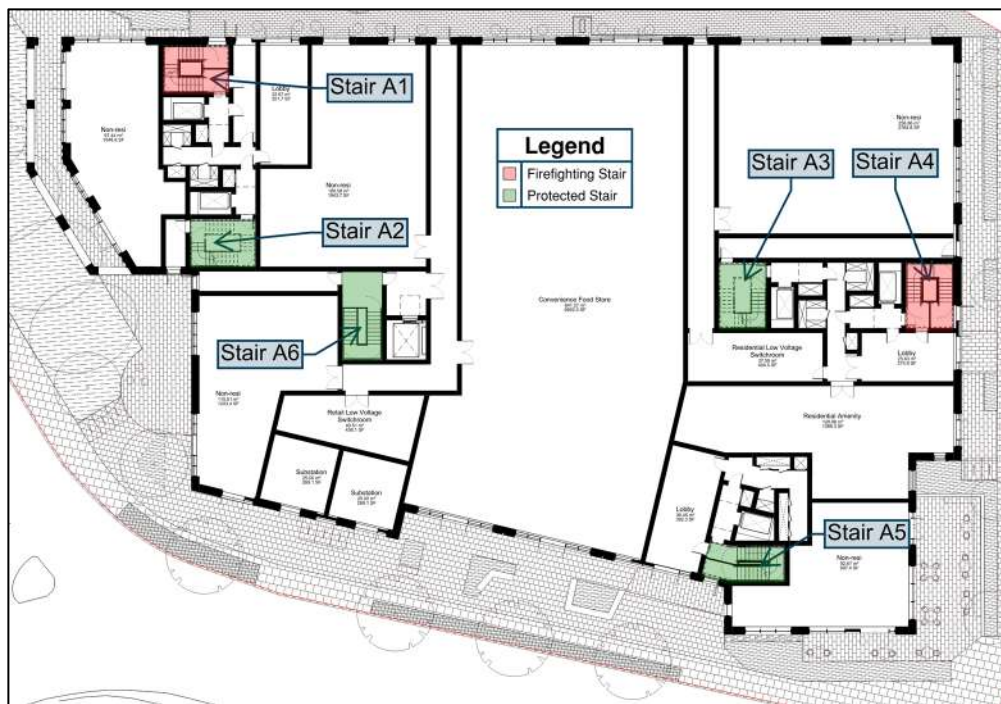
Figure 15 – Stairs Location – Ground Floor Block A
