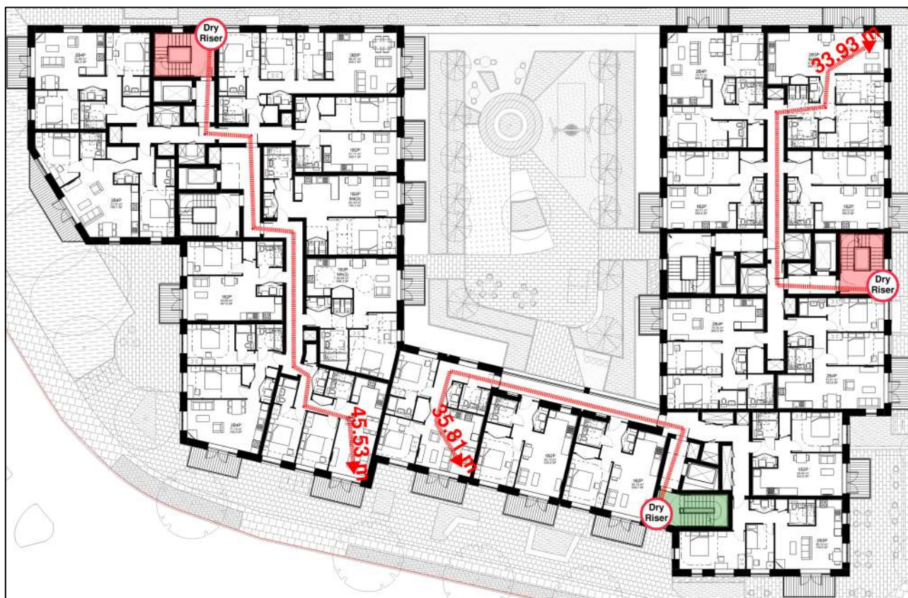
Figure 22 – Hose Distance from the Outlets – Block A
