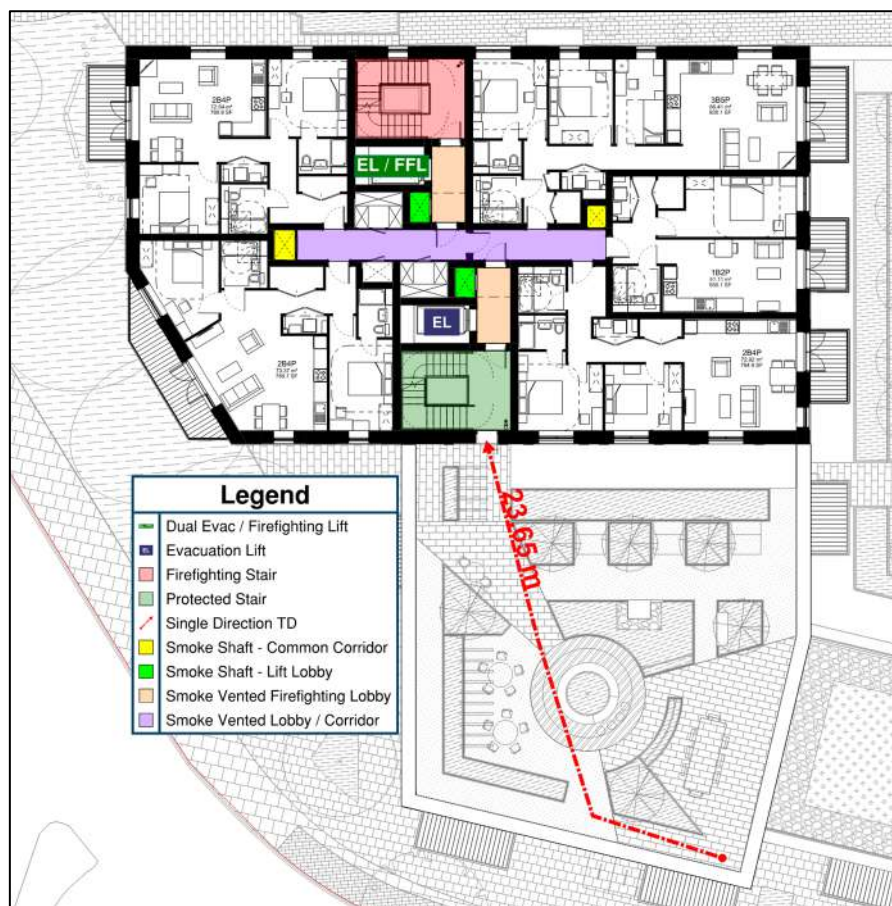
Figure 11 - Roof Terrace Travel Distance – Block A Level 06
