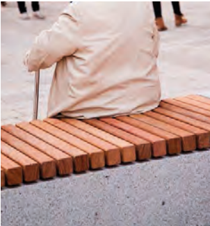
Furniture Type 01 FREE STANDING BENCH SEAT MATERIAL: STONE WITH TIMBER TOP AND METAL INLAYS SIZE: 400 (W) x 450MM (H) x VARIED LENGTH ACCESSORIES: ARMREST AND BACKREST
