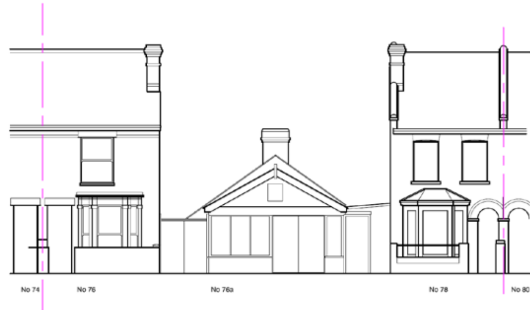
Existing elevation to Queens Road
