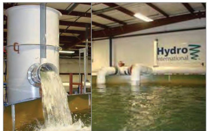
Fig.3 Grab samples were taken from the effluent discharge (pictured, left) and the influent to determine removal efficiency.
