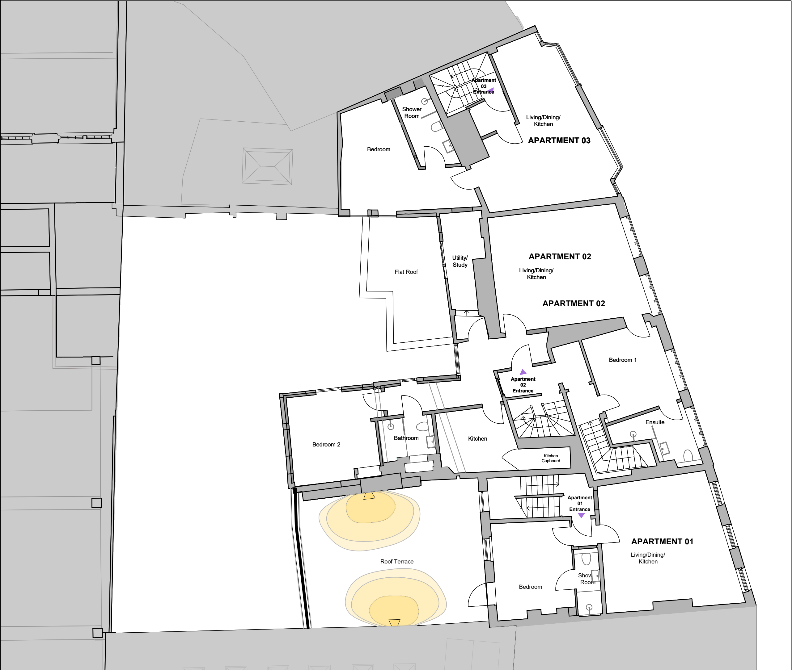
FIRST FLOOR PLAN ROOF TERRACE (EXTERNAL LIGHTING LAYOUT)
