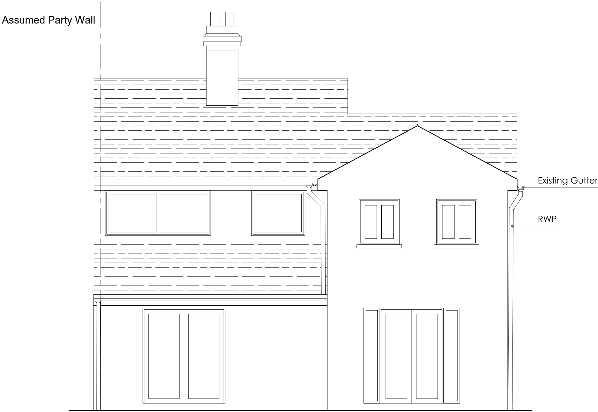
REAR ELEVATION SCALE 1:50
