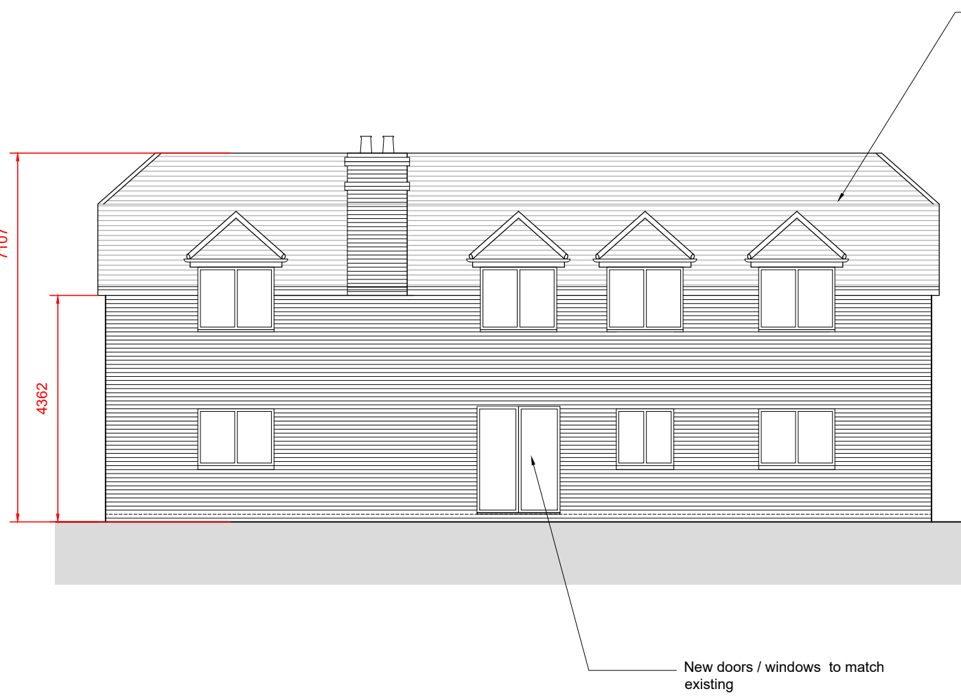
PROPOSED EAST ELEVATION SCALE 1 : 100
