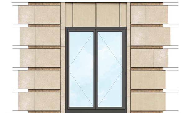
Example 2 - Existing ground floor raised fixed window in vicinity of fire escape door
