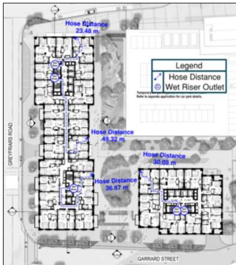
Figure 14 – Typical upper floor hose distance
