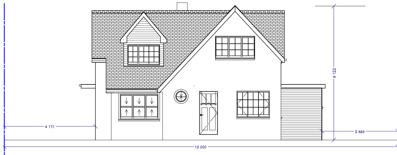
Existing Front Elevation @1:100
