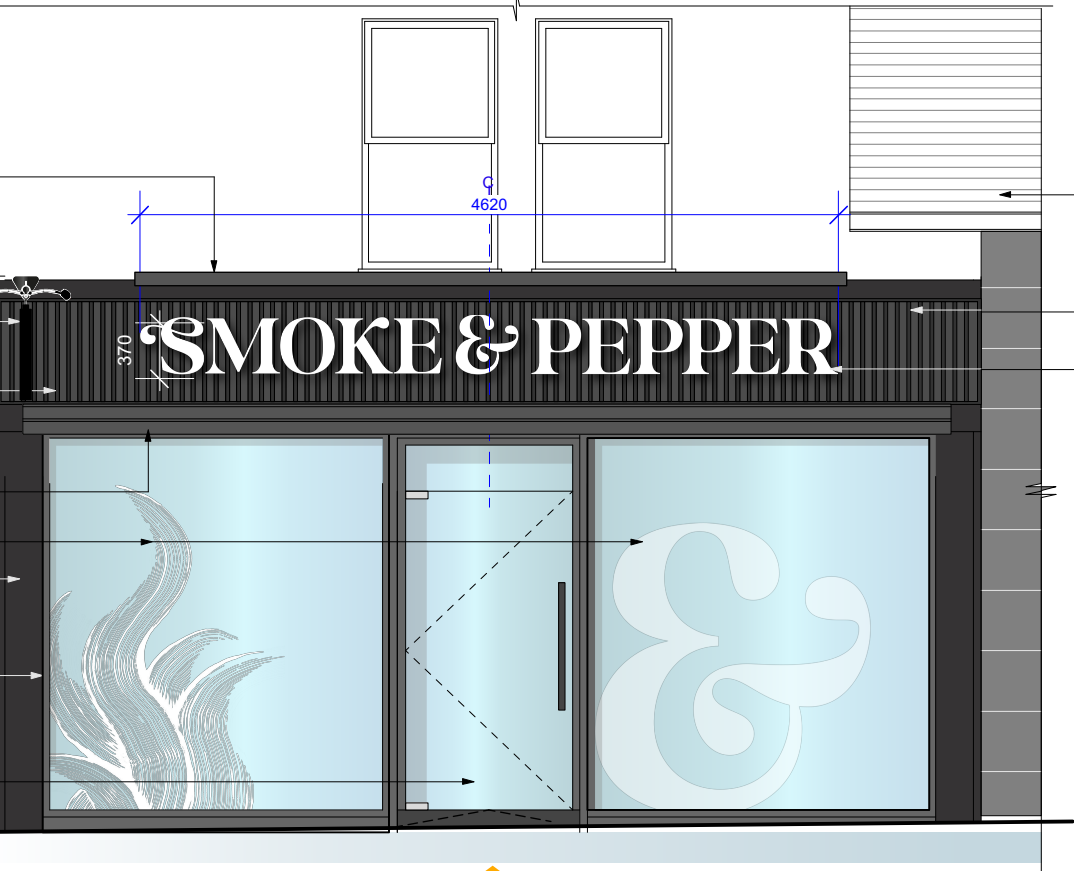
FRONT ELEVATION AS PROPOSED scale 1:50 @ A3
