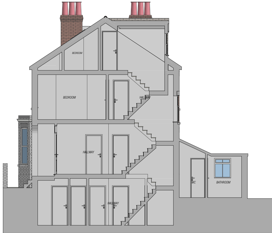
A Proposed Building Section Scale: 1:100
