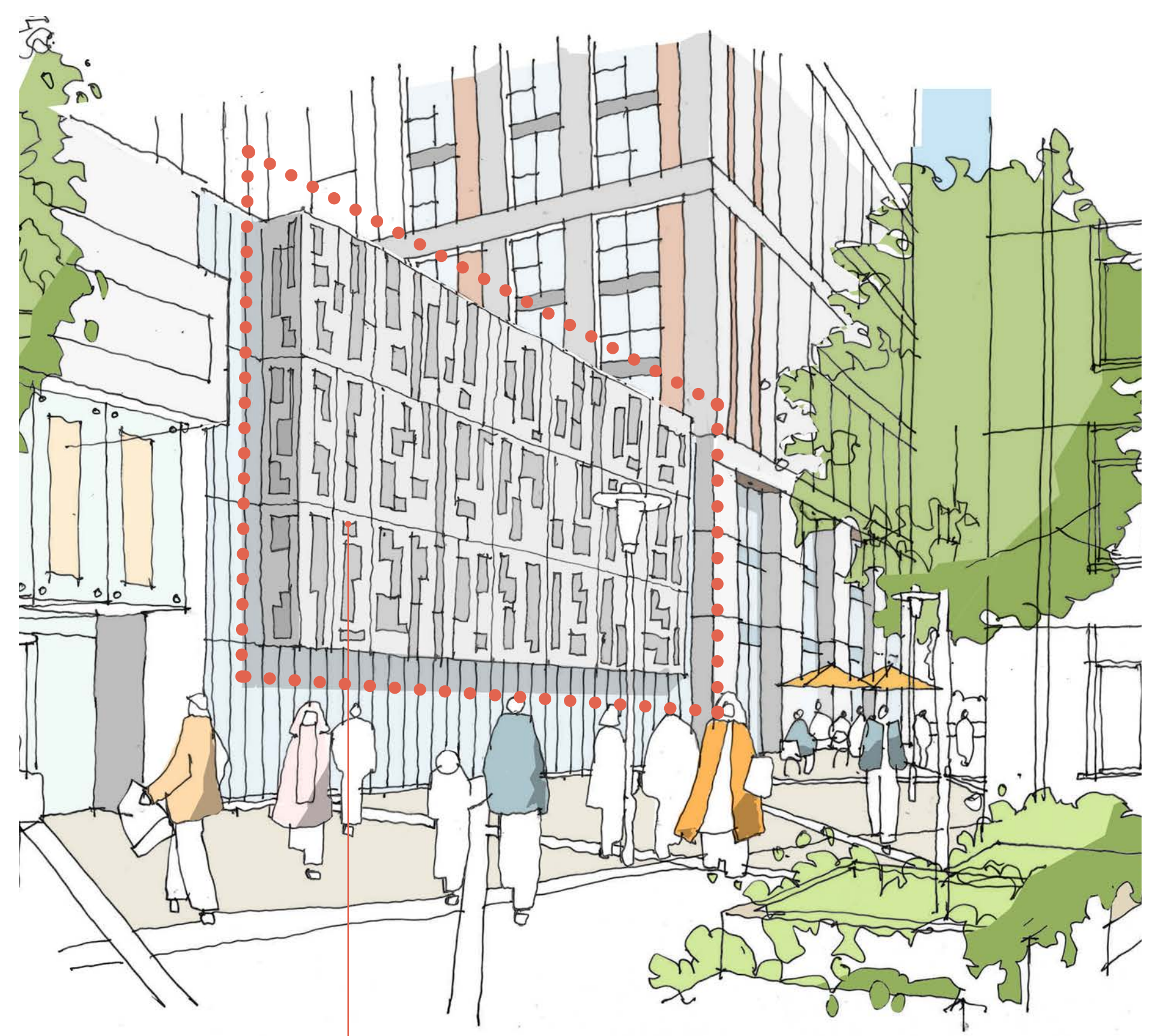
New cladding to car park ramp to use the car park frieze design in the perforations
