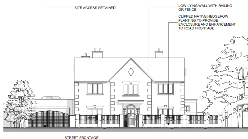
2822 004P15 Existing and Proposed Street Elevations
