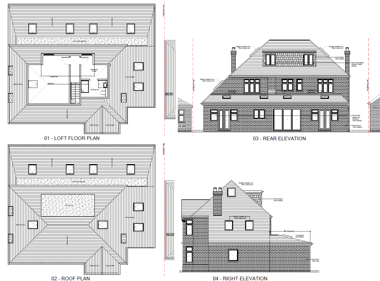
Fig. 5 Proposed Loft plans, Rear Dormer position, and Elevations
