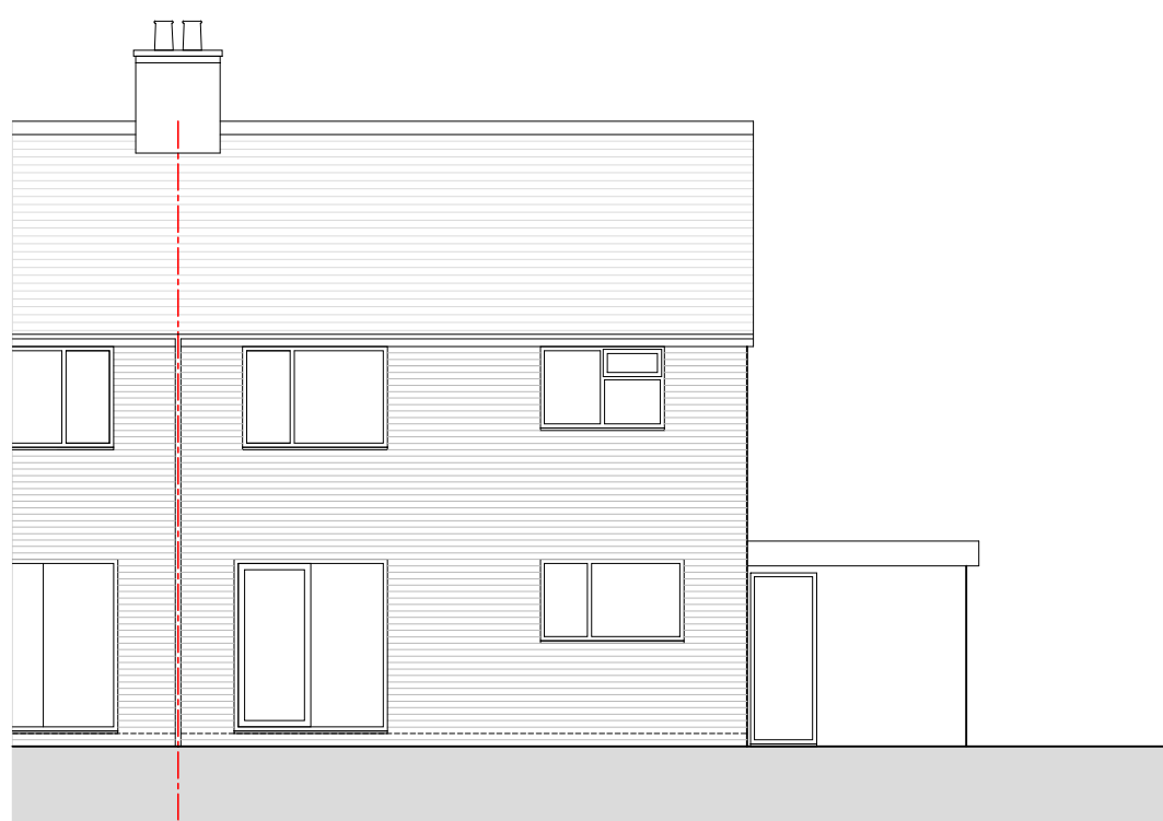
EXISTING NORTH ELEVATION SCALE 1 : 100
