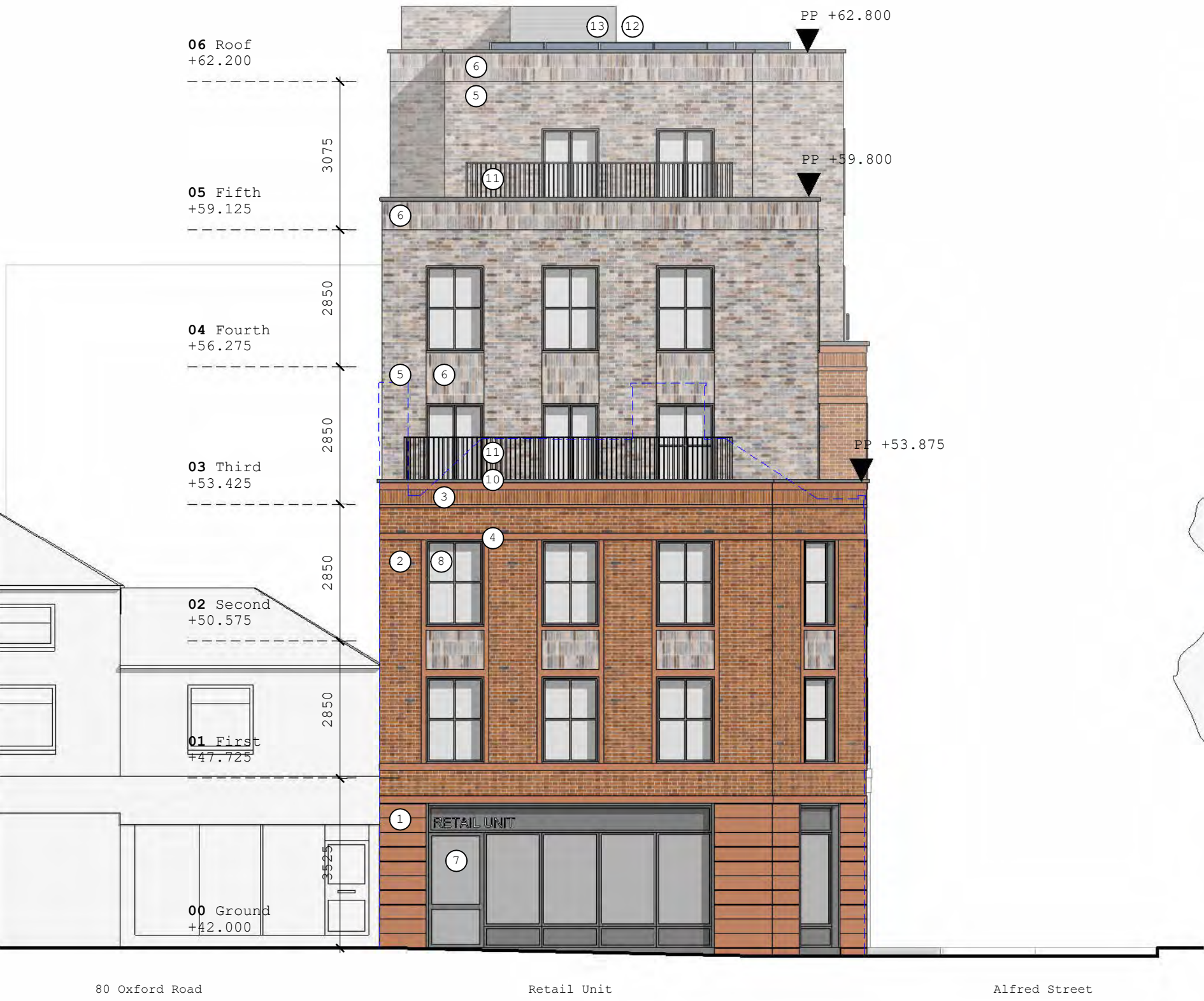
1. South Elevation (Oxford Road)
