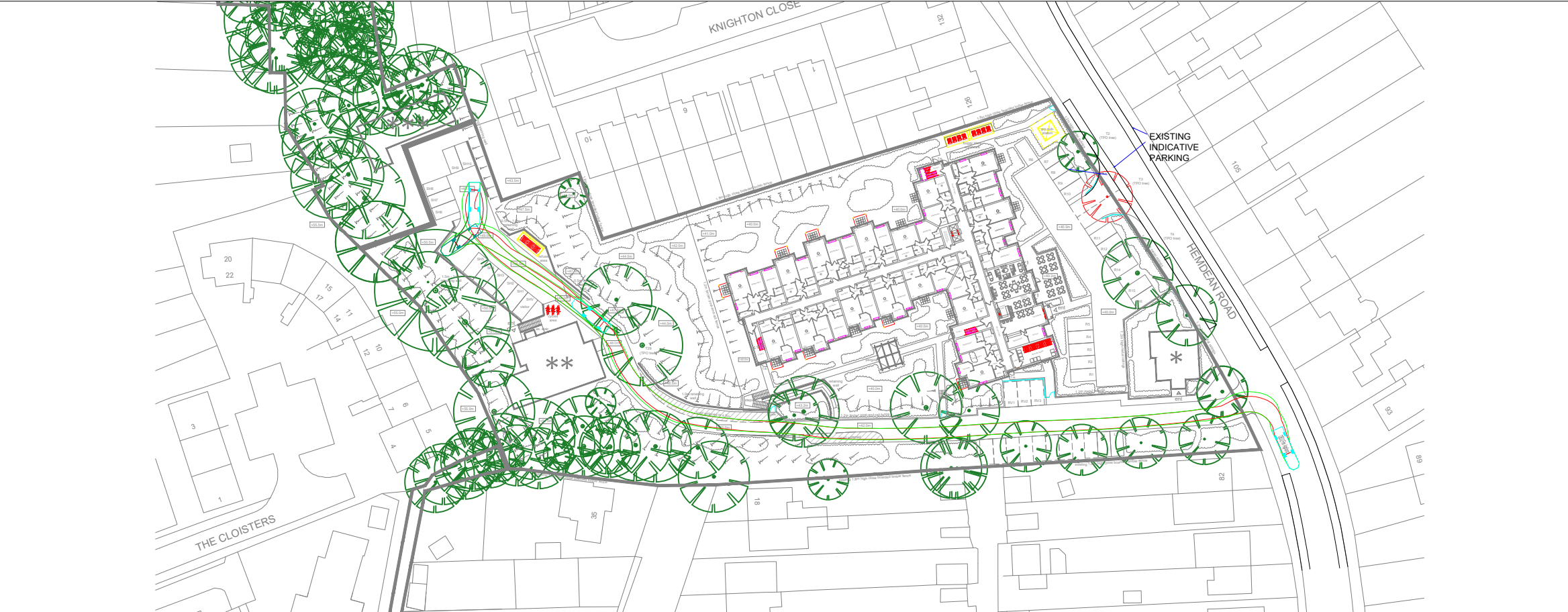
FIRE TENDER INTERNAL TRACKING 1:1000
