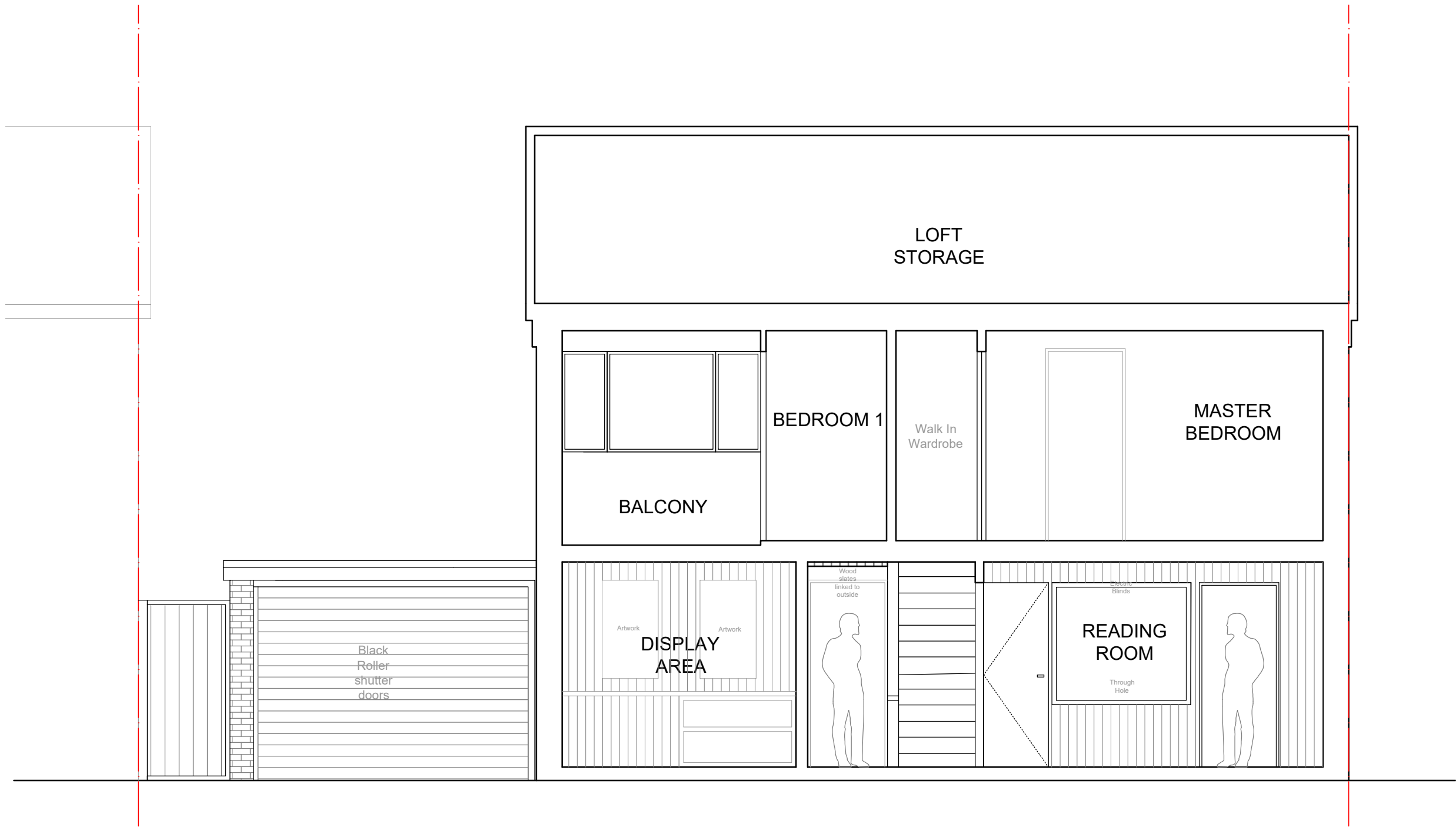
Proposed Section A-A
