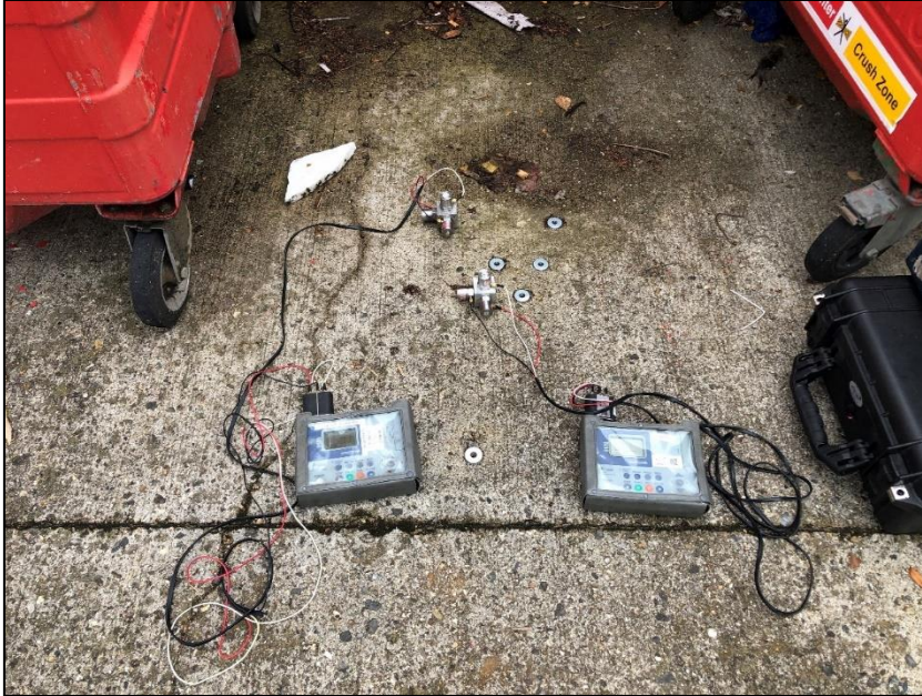
Figure 4 Vibration measurement location closest to rail tracks
