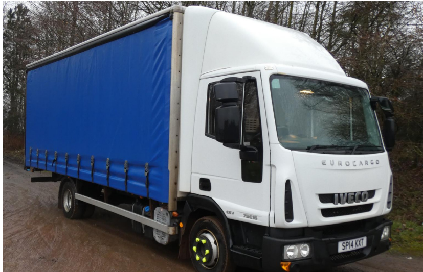
7 Tonne Curtain Waller Truck.
