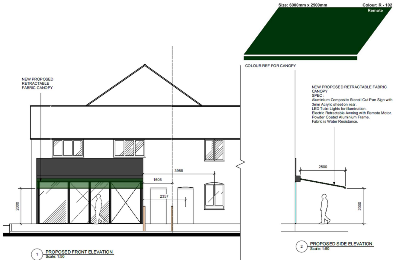
Proposed Front and Side Elevation and canopy specification
