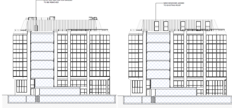
EXISTING NORTH ELEVATION (CENTRAL BLOCK)
