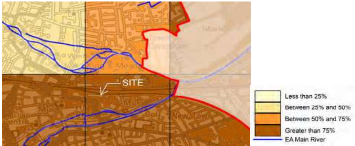
Figure 3-4: Areas Susceptible to Groundwater Flooding (Level 1 SFRA)
