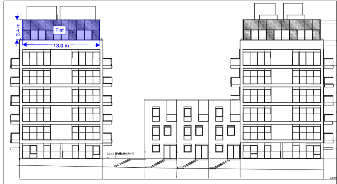
Figure 18 Southeast Elevation Worst-Case Compartment
