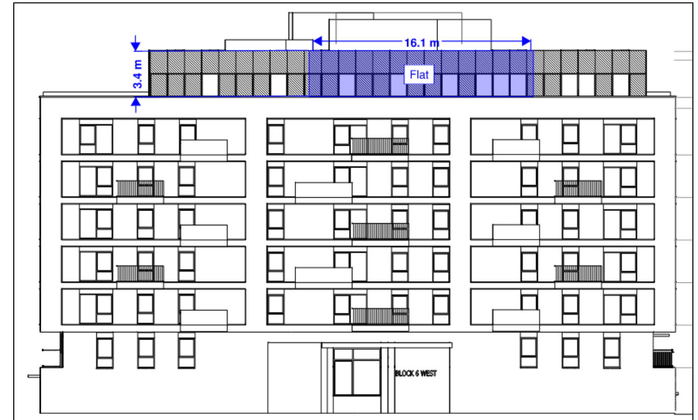
Figure 17 Southwest Elevation Worst-Case Compartment
