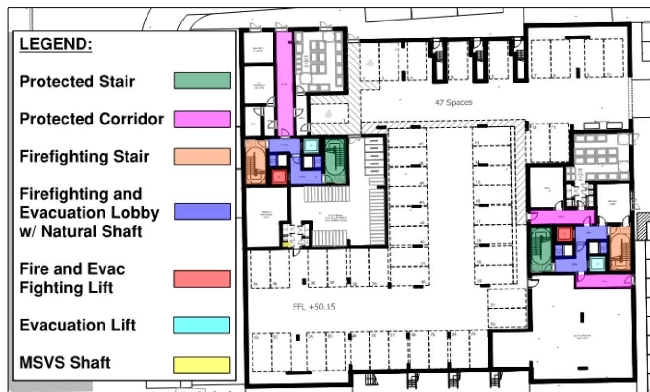
Figure 2: Lower Ground Floor General Arrangement
