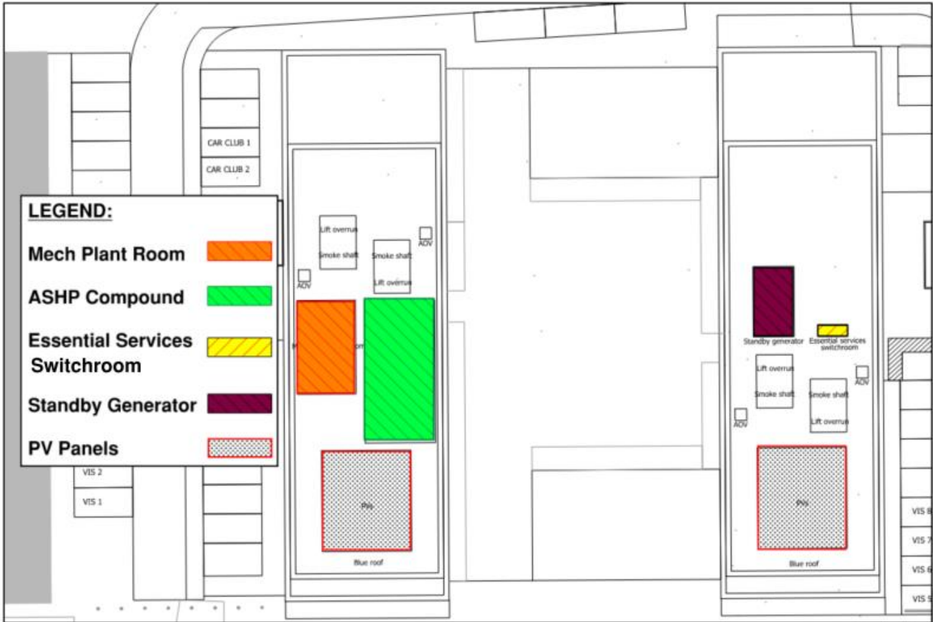
Figure 5: Roof Level General Arrangement
