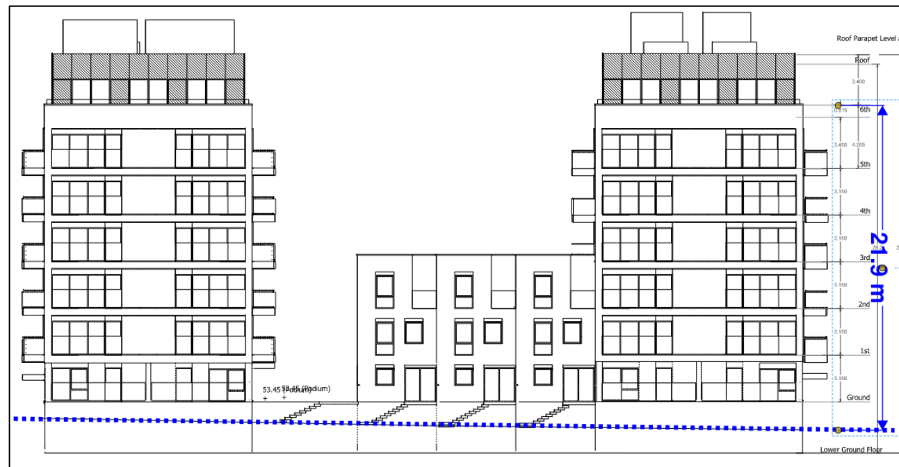
Figure 7: Southeast Elevation with Building height illustration
