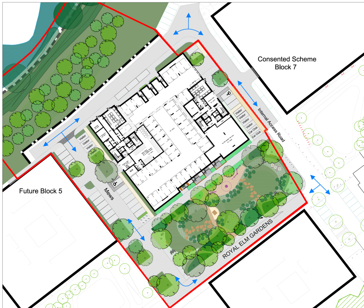
Figure 3.4: Fire and Emergency Access Routes (Block 6)
