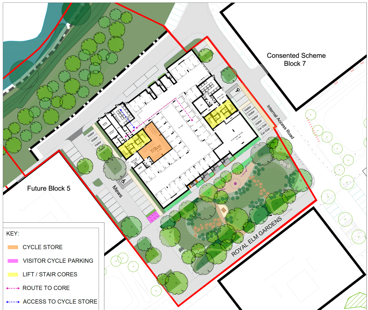
Figure 5.1: Cycle Parking Location and Access routes
