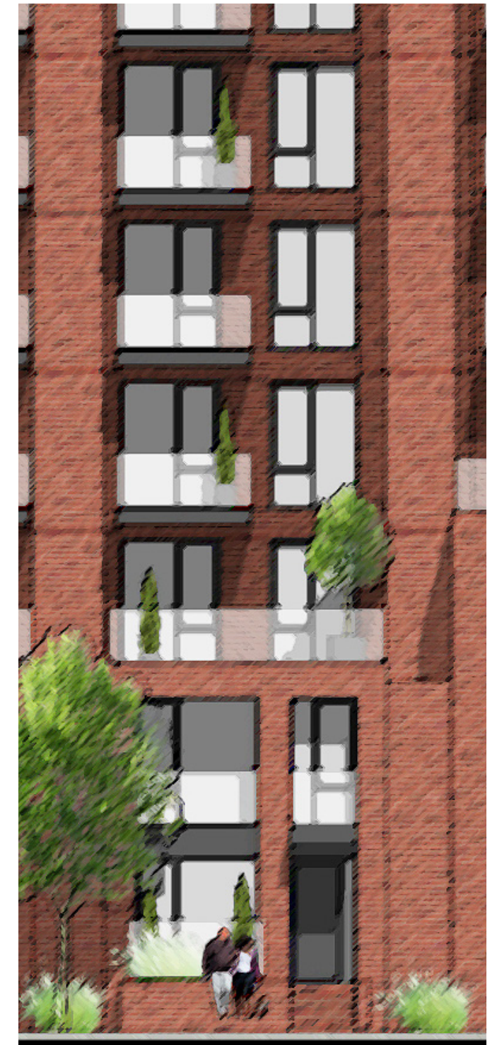
Fig. 2.23.5 - Double height articulation at street level, vertical emphasis through expression of structural piers above
