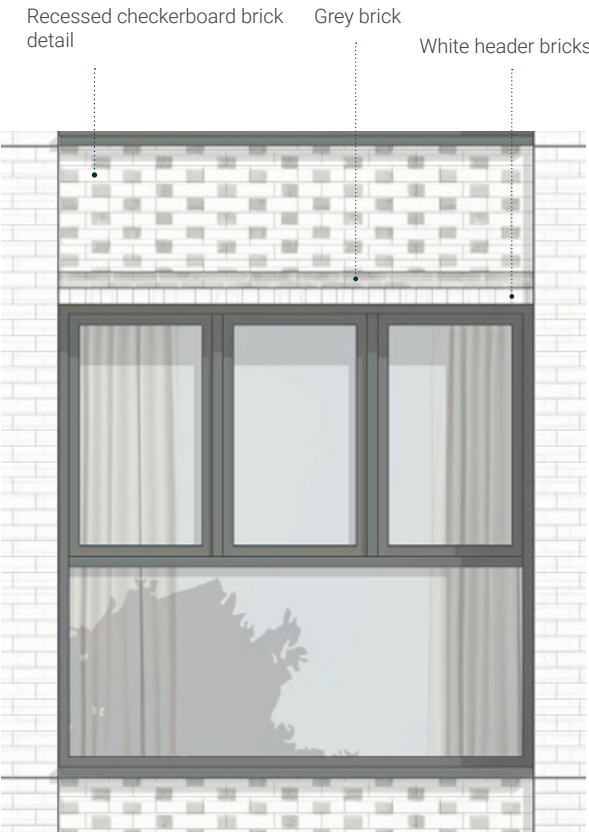
Close up elevation of window detail
