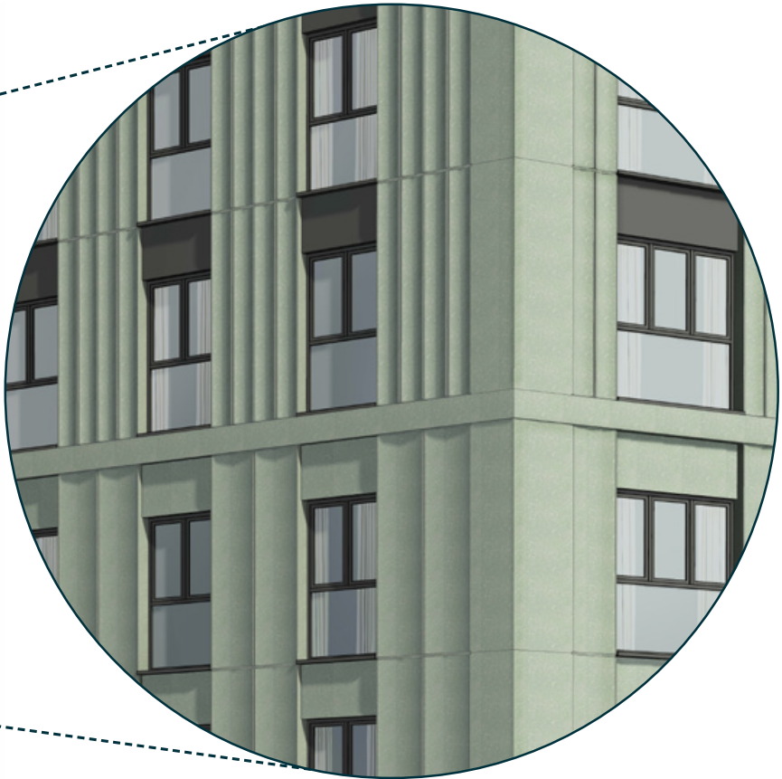
Excerpt of the facade showing the change in scale of the fluted piers, where the body of the building meets the crown
