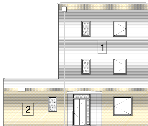
Typical elevation showing brick locations.
