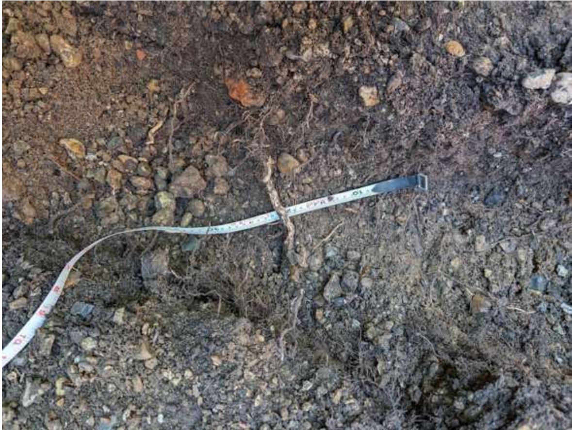
Figure 10: 2nd largest root uncovered 11mm diameter
