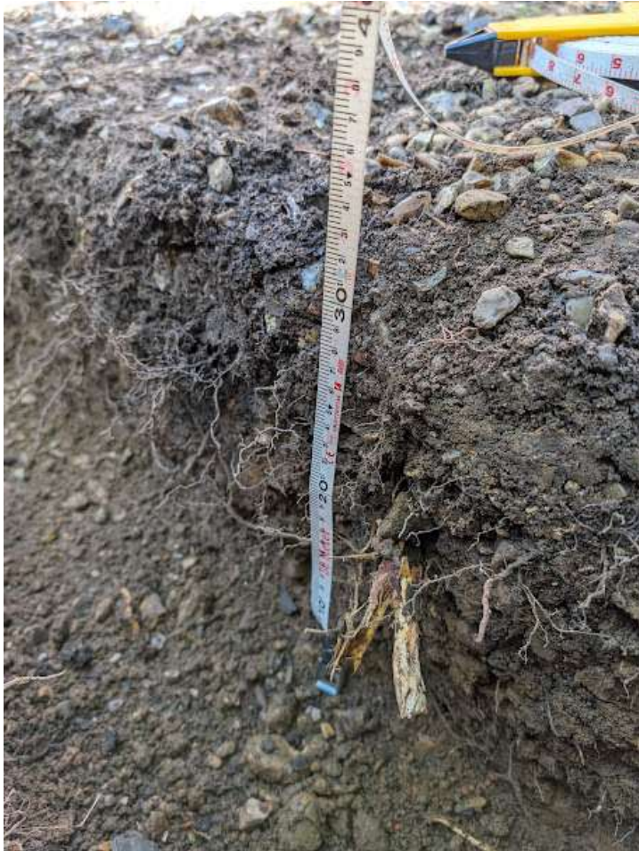
Figure 9: showing the depth of trial pit/trench 2
