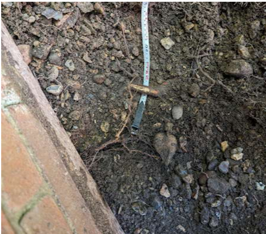
Figure 5: diameter of root 20mm
