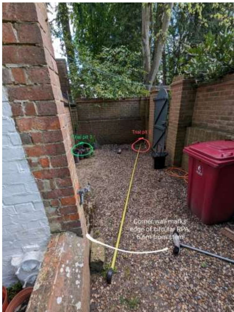
Figure 2: Annotated photo showing extent of RPA and locations of trial pits
