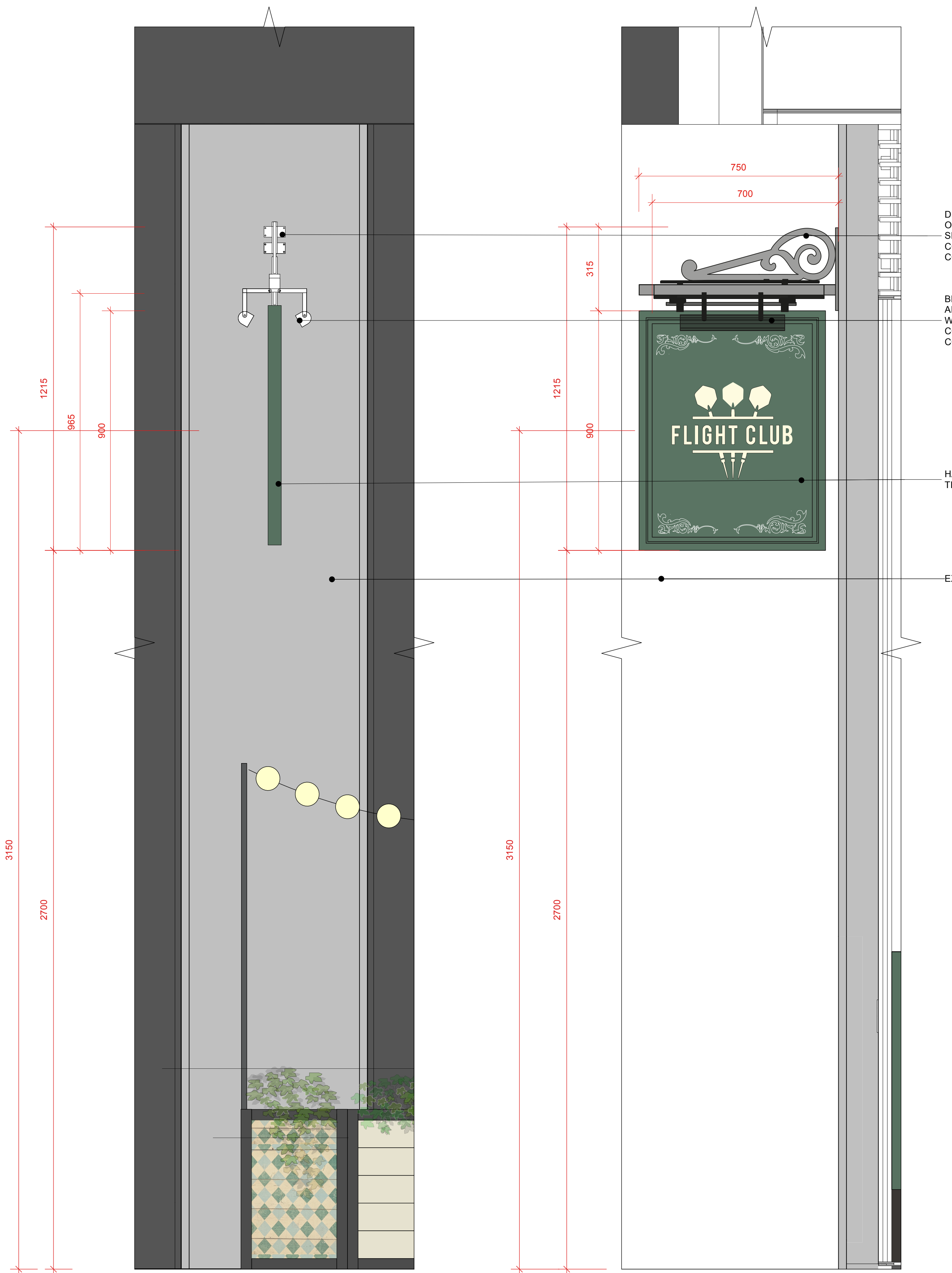
01 PROJECTING SIGN FRONT ELEVATION Scale: 1:10
