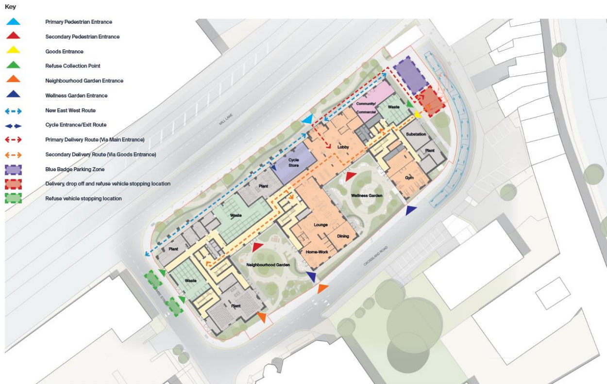
Proposed Ground Floor Plan – Access, Entrance and Servicing (page 74)
