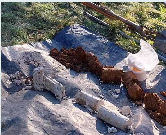
Chalk identified 2-3m bgl within WS04
