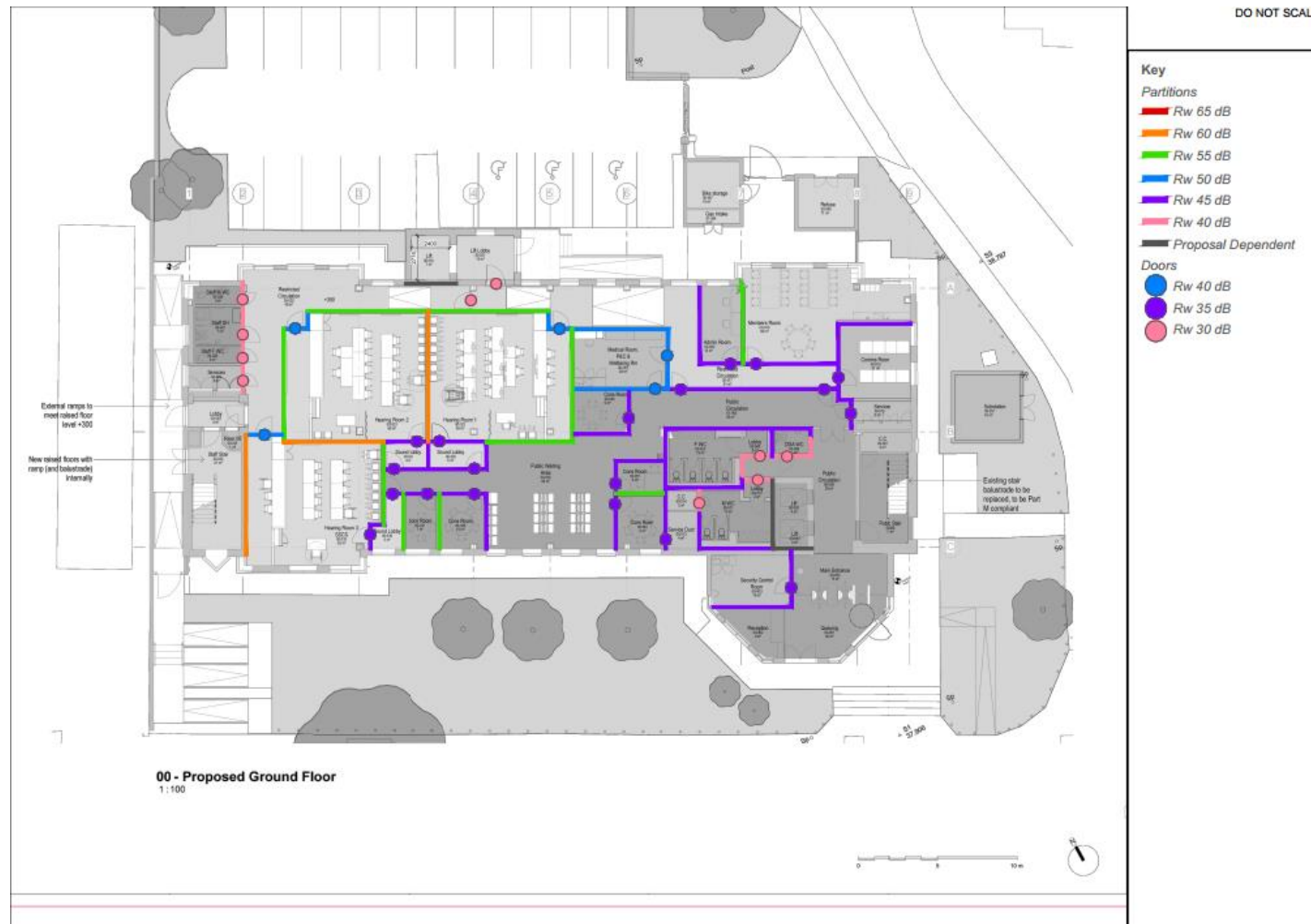
Figure C-1 Ground Floor Sound Insulation Mark-Up
